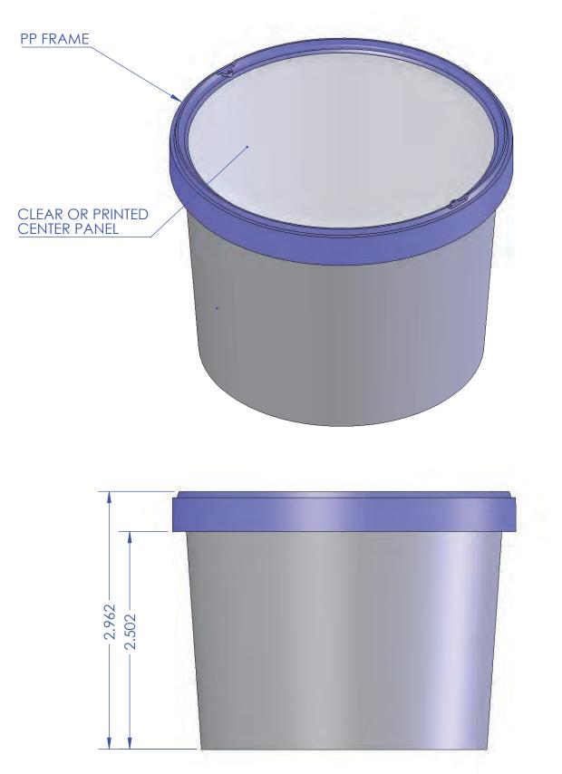
Visstun® Reusable V3™ Lid VxS2N - Clear Top VxS2F - Printed Plastic Top VxS2C - Printed Paper Top
